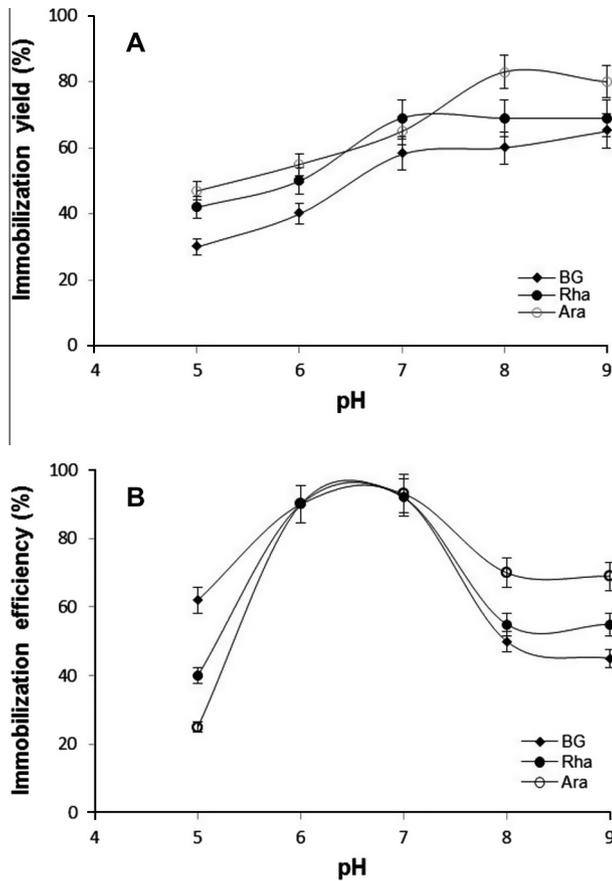
Fig. 1. Influence of coupling pH on immobilization yield (A) and immobilization efficiency (B) of the three glycosidases onto Eupergit C in 1 M sodium phosphate, after 96 h incubation time at 23 °C.
