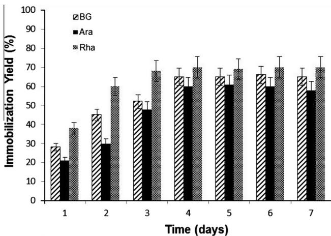
Fig. 2. Influence of coupling time on the immobilization yields of glycosidases onto Eupergit C in 1 M sodium phosphate pH 7.0 at 23 °C.
