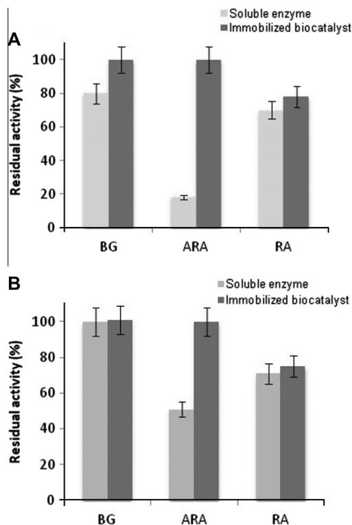
**Fig. 4.** Stability of glycosidases in model wine at pH 3.5 (A) and pH 4.0 (B), after 70 days of incubation at 23 °C. Model wine consisted of ethanol 12% v/v, containing 3.5 g/L tartaric acid, 2.5 g/L malic acid and 60 mg/L sodium metabisulfite.
