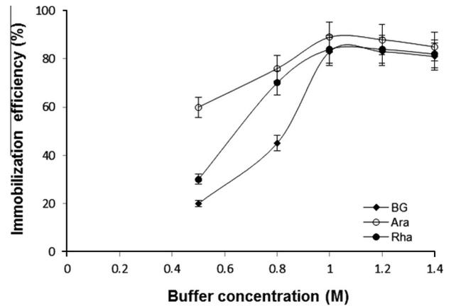
Fig. 3. Immobilization of glycosidases at different buffer salt concentrations (sodium phosphate pH 7.0) after 4 days of incubation at 23 °C.
